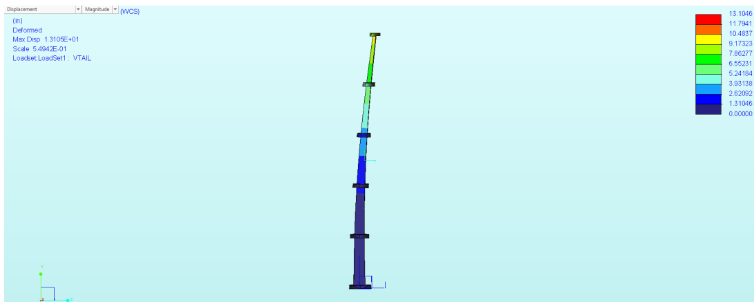
Figure 63: Deformation of the Vertical Tail Under Load
